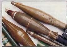
Top to bottom: product-improved PG-7 grenade with improved fuzing, ignition and motor performance; U.S. 81mm bomb mated to PG-7 racket motor; OG-7 antipersonnel fragmentation round. Standard PG-7 grenade can be identified by fluted warhead; and PG-7 boosters of assorted ComBloc origin.
